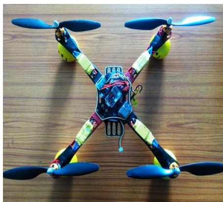
Fig: 2 Hardware assembled design of Quad copter
